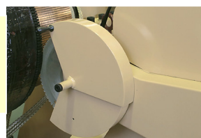
Optical sensor detects mica, controls current levels and counts bars
