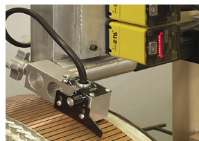
Optical sensor detects mica, controls current levels and counts bars
